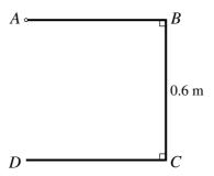
A uniform square frame ABCD has sides of length 0.6 m. The side AD is removed from the frame, and the open frame ABCD is attached at A to a fixed point (see diagram).
