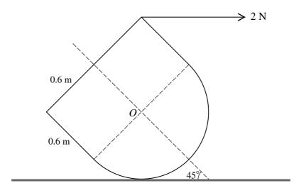
The solid is placed with the curved surface of the hemisphere on a rough horizontal surface and the axis inclined at 45° to the horizontal. The equilibrium of the solid is maintained by a horizontal force of 2 N applied to the highest point on the circumference of its plane face (see diagram). Calculate
